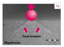
Fig. 1a) VITA ENAMIC hybrid ceramic – cross section of the fractured surface following prior damage using a tungsten carbide sphere.
