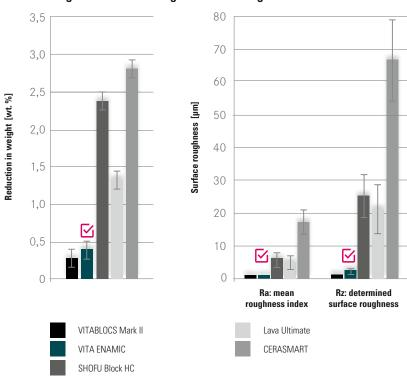
Fig. 1 Averages for weight loss and surface roughness after toothbrush abrasion on the basis of five samples per material.
