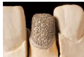
Metal framework after sandblasting with aluminium oxide
