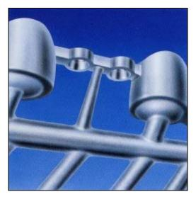
When using bars it is also important to position an extra casting sprue in the middle to obtain an optimal result.
