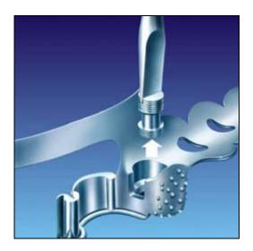
After casting remove the threaded core, used as a spacer. However the nut should be covered with wax during electrolytic polishing, in order to avoid damage. Finish as usual.
