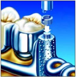
After finishing the cast frame place the male into the female and then position the frame onto the model. After that tighten the male from above using the open nut.
