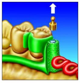
Before wax up remove the brass cap and cover the castable nut with wax. It is important to position the sprue approx. away from the nut. When you adapt the sprue directly onto the nut, it is possible that the penetrating metal can make the nut shrink during cool down.
