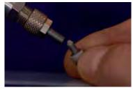
Sandblast the bonding surface of the Ti abutment with  $50 \, \mu m \, Al_2O_3$  and maximum 2 bars maintaining around 1 cm distance from the abutment.
