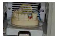
Light cure each side for 20 seconds with a Halogen/ LED lamp with minimum of 700 mW/cm2 (wavelength between 430 and 480 nm).
